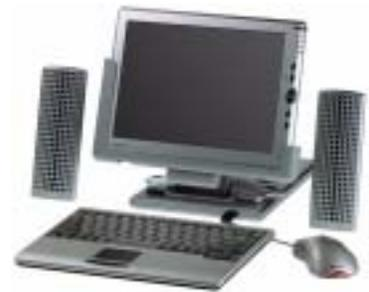
The Motion Tablet PC display, unlike touchscreens and personal digital assistants (PDAs), responds to the Motion Digitizer Pen, but not to a PDA stylus or to finger taps.
